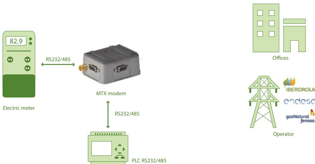
EXAMPLE 2. Remote 3G access to RS232/RS485 serial devices. Modes TCP server, TCP client and UDP
